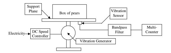
Figure 1. Vibration device for inducing skin browning on pears.
